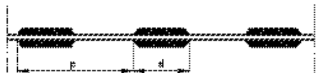
Figure 1 : Intermittent chain welding
